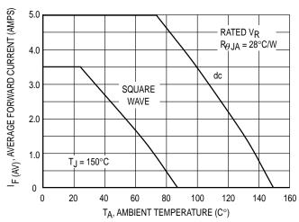
Figure 3. Current Derating Ambient (Mounting method #3 per note 1)
