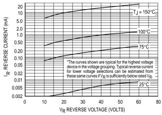
Figure 2. Typical Reverse Current\*
