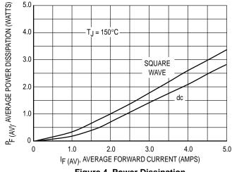
Figure 4. Power Dissipation
