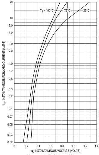
Figure 1. Typical Forward Voltage
