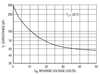
Figure 5. Typical Capacitance
